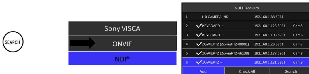
After the search is completed, use the up, down and top button of the joystick to select the camera to add. A " ✓ " sign will appear in front of the selected camera .
