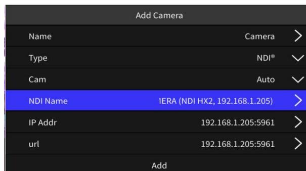
Select the type as NDI, and the Cam number can be specified or automatically assigned in the order of addition.
